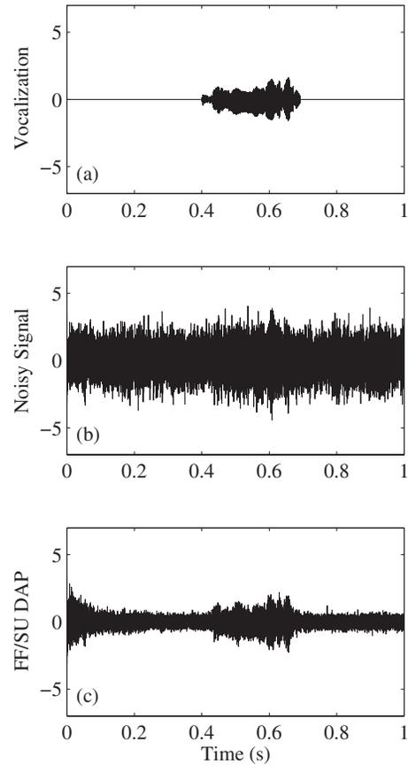
FIG. 7. (a) A clean manatee vocalization in the time domain, (b) the noisy measurement with input SNR equal to  $-5$  dB on channel 1, and (c) the time domain output of the FF/SU DAP algorithm (plots are for the channel 1 measurements; the input SNR for channel 2 is  $-13.4$  dB).
